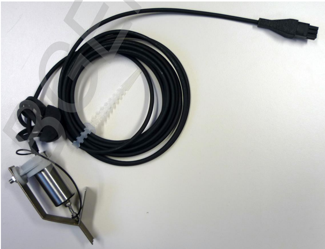
Picture 13: Diameter variation sensor
