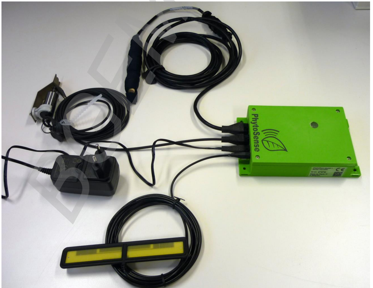
Picture 11: PhytoStem data logger with accessories
