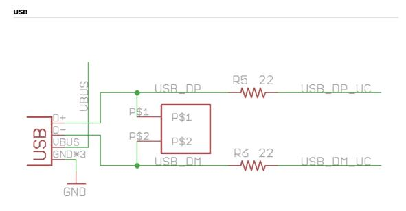
The USB data lines are terminated with 22 Ohm resistors. These data pins are also exposed via small through holes next to the USB connector and are labeled D+ and D-. The VBUS (+5VDC VCC of the USB port) is fed to the PMIC via a 3Amp Schottky diode (<u>SS3P3</u>). The VBUS pin is also available via the unpopulated header hole on the top-right side of the Electron.
