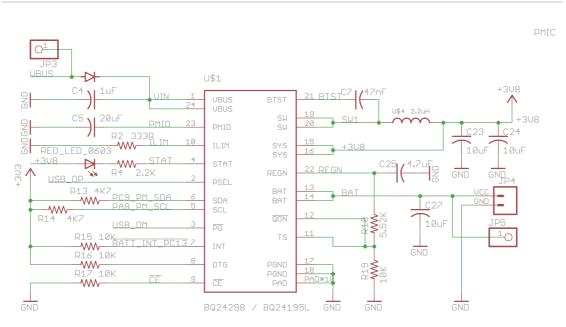
The Electron uses TI's <u>BQ24195</u> as the power management and charging unit. This PMIC intelligently sources power from either the VIN pin, the USB port and/or the LiPo battery. When all the power
