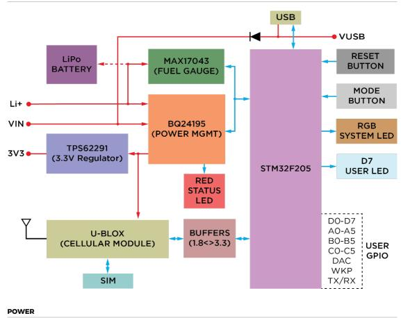
The Electron can be powered via the VIN (3.9V-12VDC) pin, the USB Micro B connector or a LiPo battery.
