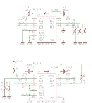
Since u-blox module's communication interface operates at 1.8VDC, while the STM32F205RGT6 microcontroller operates at 3.3VDC, we need voltage translators in-between them. This is achieved with two <u>SN74AVC4T245</u> non-inverting buffers. The default state of the USART pins is set with the help of pull-up and pull-down resistors, and the unused input pins are tied to GND.
