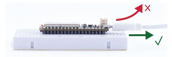
The u.FL antenna connector is a very fragile piece of hardware ( and is fancy too with all the gold plating). The connector was not designed to be constantly plugged and unplugged. Care must be
