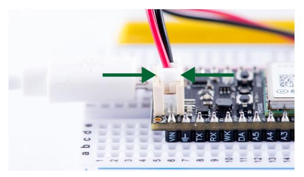
The micro B USB connector on the electron is soldered on the PCB with large surface pads as well as couple of through hole anchor points. Despite this reinforcement, it is very easy to rip out the connector if too much stress is put on in the vertical direction.
