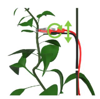
Fine-tune the sensor positioning by bending the wire and/or rotating the sensor around the wire.
