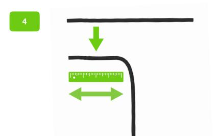
Bend the sensor positioning wire in an L-shape using the measured distances.
