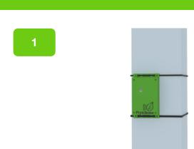
Firmly secure the PhytoSensor data logger to the greenhouse structure. E.g. using cable ties going through the holes in the enclosure.
