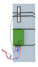
Connect the sensor cables to the data logger.
